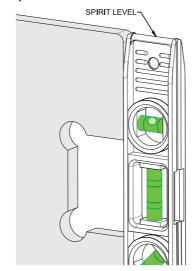
**3.** Ensure that all the glass panels are plumb and level. Also ensure that the hinge panel is securely fixed to guarantee the hinge panel stays plumb.
