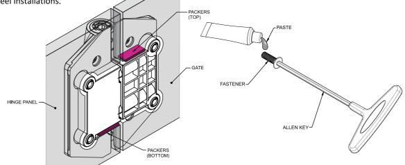
5. Using blocks + packers, place gate into position with extra 2mm higher at the latch end to allow for glass weight droop. Once gaps and packers are in the correct positions, screw the fascia plates with the gaskets into place. Hinges are to be fitted straight and parallel to each other.
