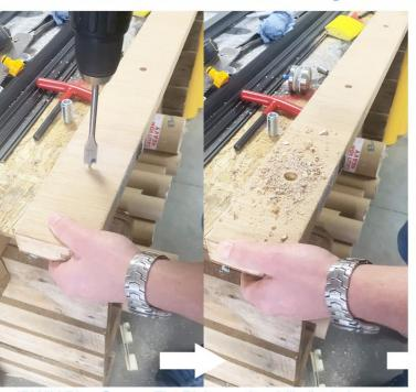
IRWIN Blue Groove Flat Bit is used to drill pilot holes
