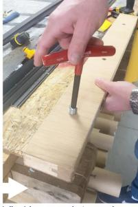
Secure using a 10mm hex (allen) key or socket wrench.
