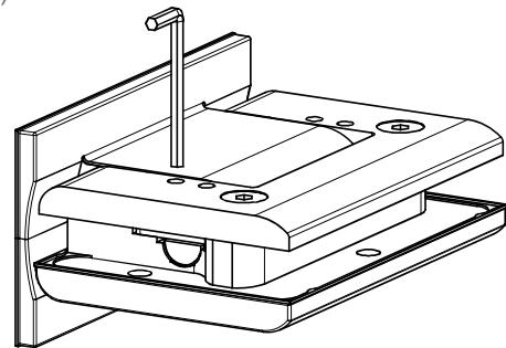
Hydraulic hinge with adjustable closing speed of the door. Suitable for both internal and external doors. The inner body is fully anodized with high thickness special oxidation treatment (20 microns). The outer covers are made of stainless steel AISI 316, both polished and satin finish. Stop at 0°+ 90° -90°. Glass thickness: 8 -13.52 mm.
