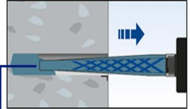
Insert anchor injection resin. (Clean again with air pump to achieve the perfect fixing surface)
