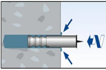
Insert anchor - Rotate to achieve a solid fixing.
