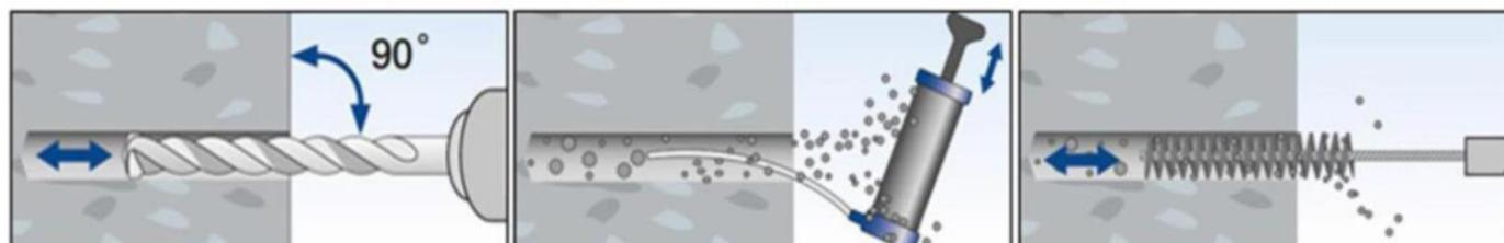
After drilling the correct size fixing hole and cleaning with air pump to remove dust and debris.
