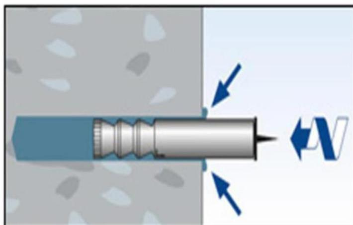
Insert anchor - Rotate to achieve a solid fixing.
