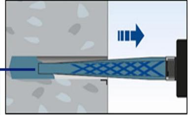
Insert anchor injection resin. (Clean again with air pump to achieve the perfect fixing surface)
