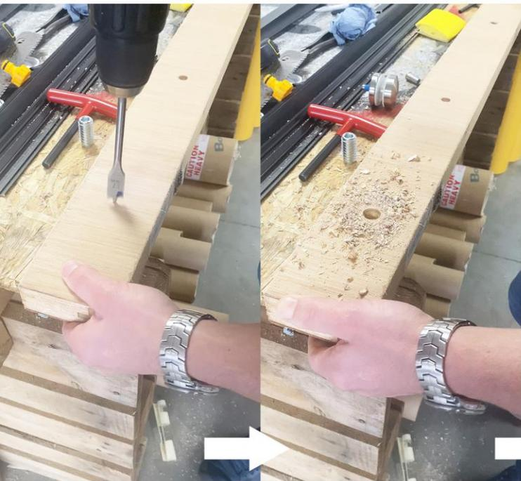
IRWIN Blue Groove Flat Bit is used to drill pilot holes
