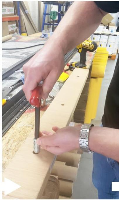
Secure using a 10mm hex (allen) key or socket wrench.
